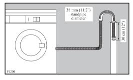
When discharging into a standpipe ensure that the top of the standpipe is no more than 90cm (35.4") and no less than 60cm (23.6") above floor level.
